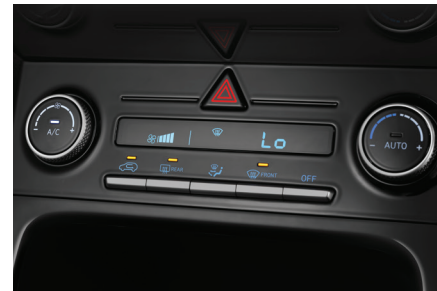
Full Automatic Temperature Controls
